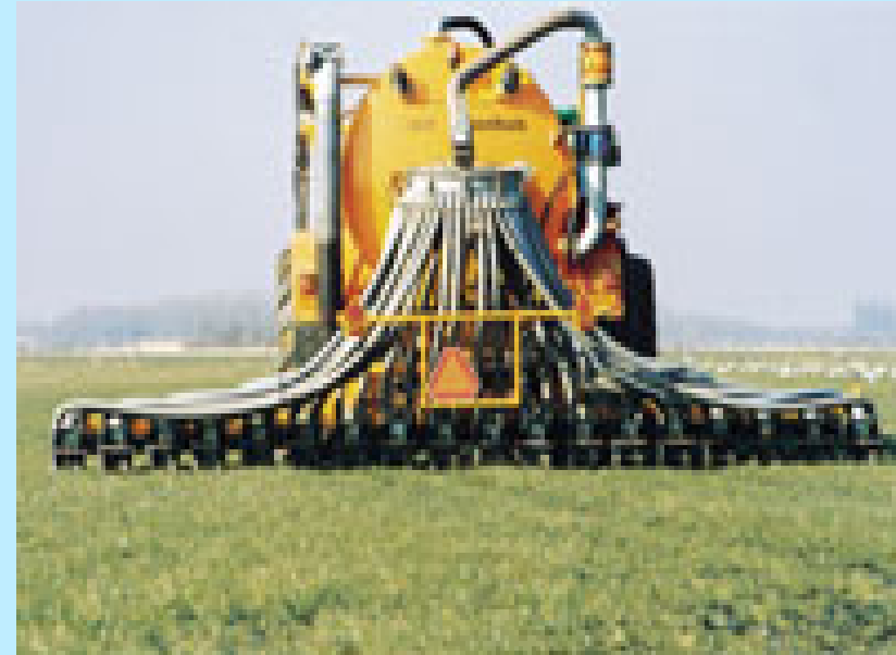
Injection into the soil of liquid animal manure
